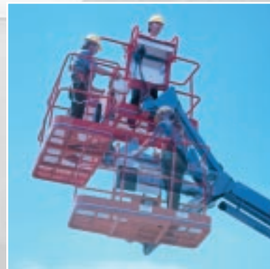
180° powered platform rotator , which functions regardless of jib location.
