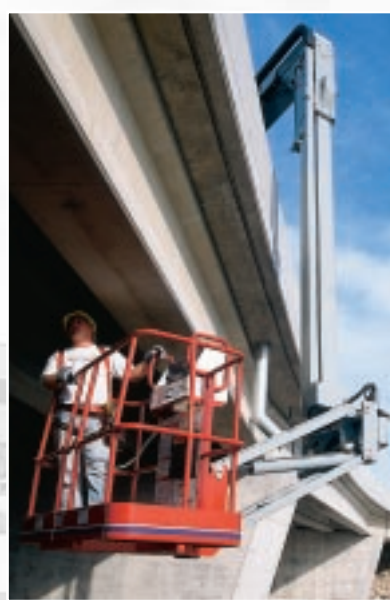
Optional Feature: Exclusive rotating jib option increases reach to work around obstacles. The rotating jib is capable of a 90° turn in either direction from center.
